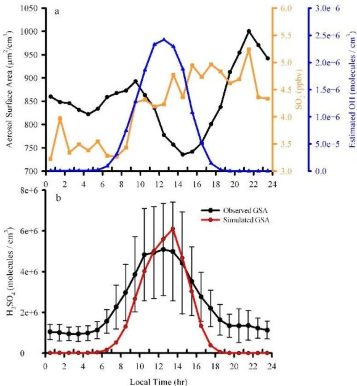
Gaseous  $\text{H}_2\text{SO}_4$  (GSA) can initiate new particle formation and, upon uptake, significantly modify pre-existing aerosol's morphology, hygroscopicity, and optical properties. In-situ measurements of GSA is fundamental to fully comprehend the evolution of aerosol in the atmosphere and its interaction with solar radiation. From 7 July to 25 September 2008, Drs. Jun Zheng and Renyi Zhang from the Texas
